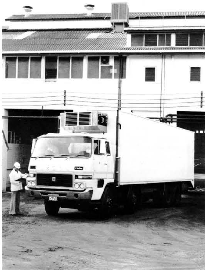
New Isuzu SPH 710 can cope with heavy loads, with tandem axle and twin-steer.
